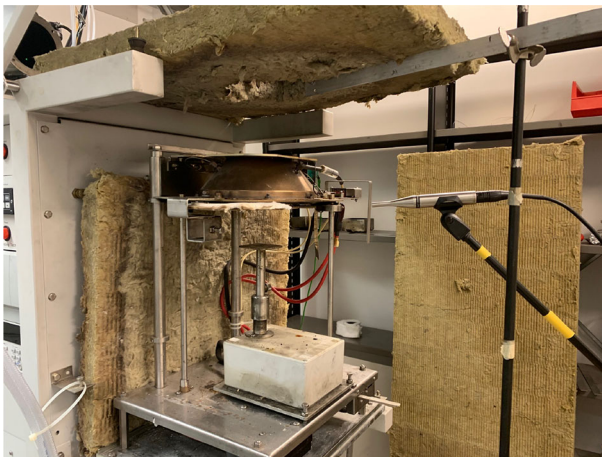
Figure 2. The cone calorimeter setup used in the experiments.
